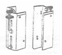
Use ½" diameter stainless steel bolts with stainless steel lock nuts for installation. Over sized washers should be used inside transom to prevent damage.
