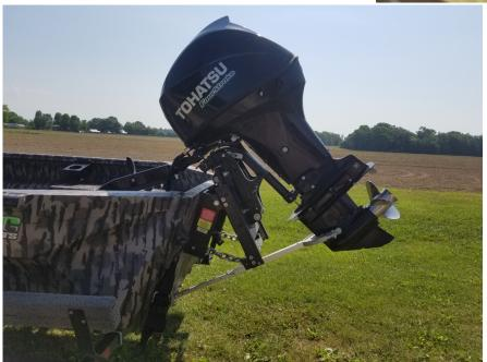
4. The chains are fully extended and the engine does not move up or down. Also, lock your engine steering mechanism if your unit is a tiller handle engine. This will prevent your engine from moving side to side possibly damaging your engine saver.
