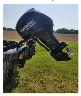
2. Install your engine saver bracket so that the engine is resting on the engine saver bracket. This part is required for safe trailering operation, we do sell engine savers separately on <a href="https://www.vancemfg.com">www.vancemfg.com</a>, contact us if you are not sure what length engine saver bracket you need.
