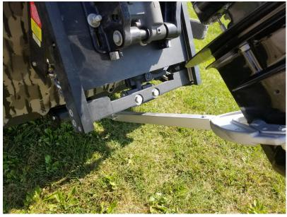
Ensure your engine saver is not impacting your kick-up plate operation on the bottom of your unit.
